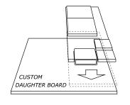
Warp with application specific peripherals using a traditional MCUs as a sensor hub. This differs from traditional carrier boards since Warp is fully self contained.
