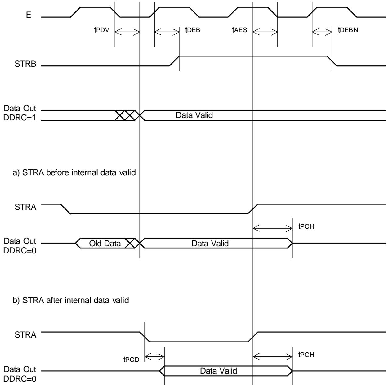
Figure 9. Port C Three-State Output Handshake Timing
