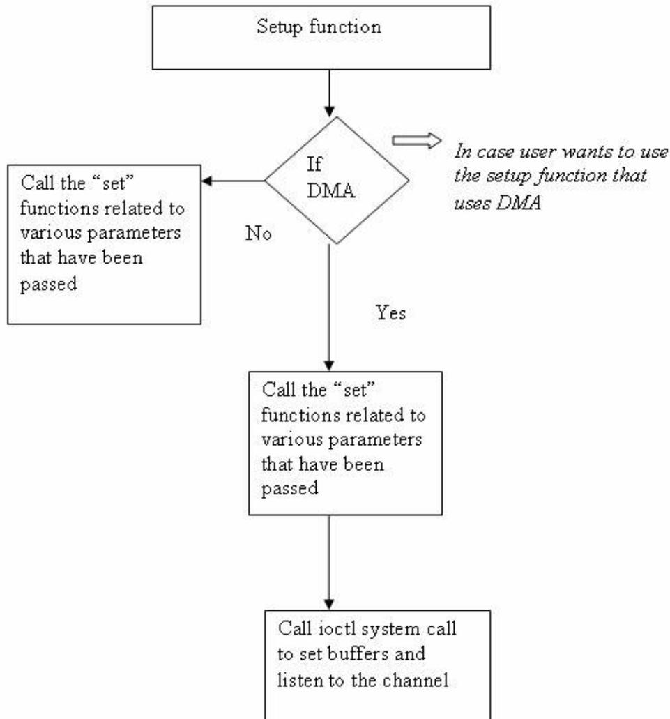
As shown in Figure 3, the Setup function in turn calls various set functions to set the parameter values to the camera registers. In the case of DMA setup, after the set functions have been called the ioctl system call is called to set the DMA buffers.
