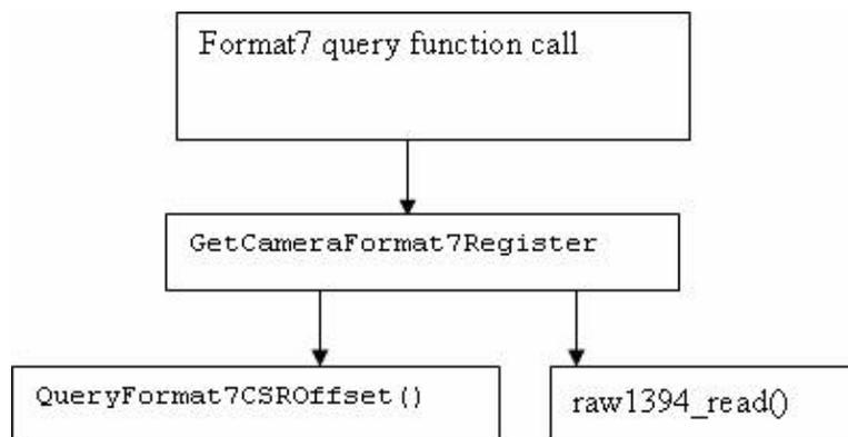
The Format7 query function will call `GetCameraFormat7Register`, which is supposed to read the values from the control and status registers of the camera. This function in turn will call the `QueryFormat7CSROffset` and `raw1394_read` to know the offset for the particular information that has been queried. After getting the offset, `raw1394_read` is used to actually read the values.
