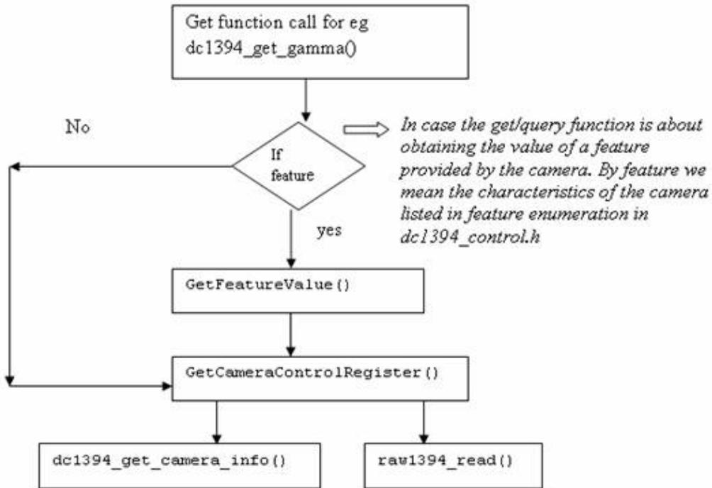
In case the `get` function you called is meant to retrieve the value of a camera feature (the value for the parameters listed in feature enumeration), that `get` function will call another `get` function (`GetFeatureValue`), which takes the enumeration value of the feature as input. For example, in the case of gamma value, the function passes 422 as the value (this value can be calculated from the enumeration given in the `dc1394_control.h` file).
