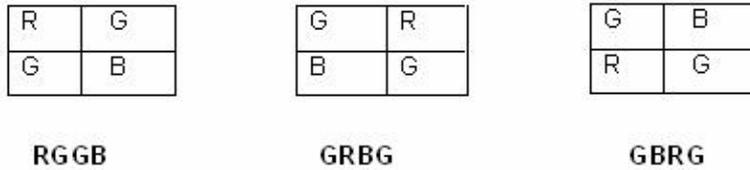
The image we obtained in the previous example was a Bayer Pattern image also known as a *RAW* image. This was stored in `camera.capture_buffer`. In order to view what we have captured we convert this *RAW* image to *.PGM* by adding a header (look at the explanation in [Section 4.4](#)).
