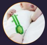
A Kimono\* with sensors monitors the baby's temperature, breathing and communicates with parents.
