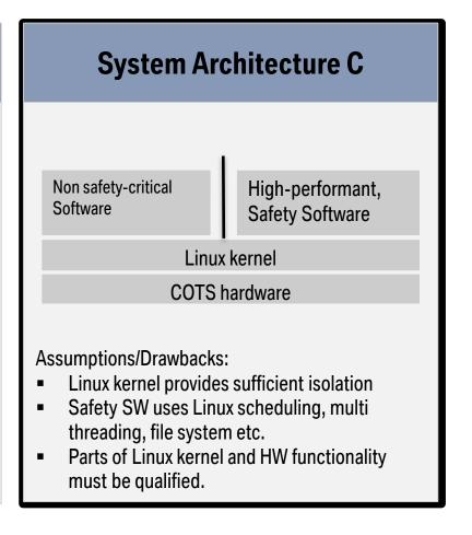
SIL2LinuxMP Project focusses on work for system architecture C.
